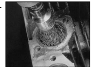
Cleaning the exhaust port of a gasoline engine.
